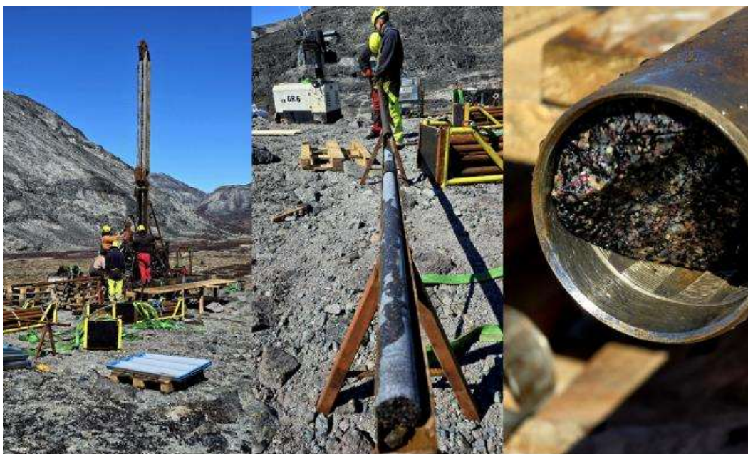
Figure 4 – Drill hole 26-02, drill core from the hole, strong eudialyte containment.
